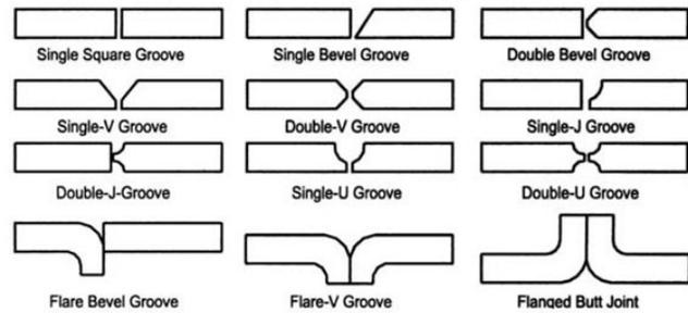
Figure 4: Butt Joint Weld Configurations
