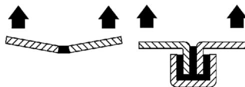
Figure 6: Cleavage Joint Redesign
