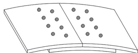
Figure 1: Riveted Butt Splice Joint
