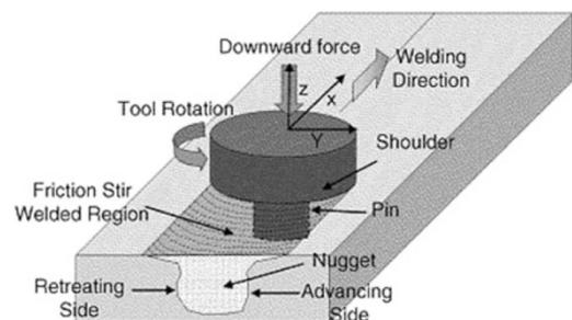
Figure 3: Friction Stir Welding
